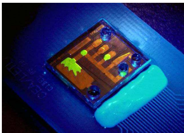
Figure 8: Diagram and photo of closed EWOD chip.
