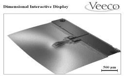
Figure 1. Gauge deformation due to thin film stresses.
