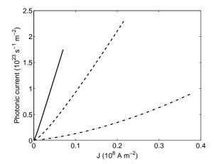
FIG. 4: Photonic current density versus electronic current for different values of the intersubband transition energy:  $E_{12} = 50 \mathrm{meV}$ , (dashed-dotted line),  $100 \mathrm{meV}$  (dashed line) and  $150 \mathrm{meV}$  (solid line). Same parameters and range of applied voltages as in Fig. 3.
