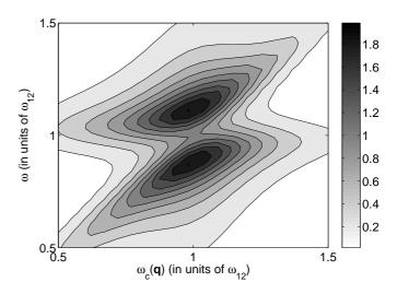
FIG. 8: Contour plot of the electroluminescence (arb. units) as a function of the bare cavity photon energy  $\omega_c(q)$  and of the emission frequency  $\omega$  for an applied voltage  $eV=0.5E_{12}$ . The anticrossing of the two intersubband polariton branches is apparent in electroluminescence spectra.
