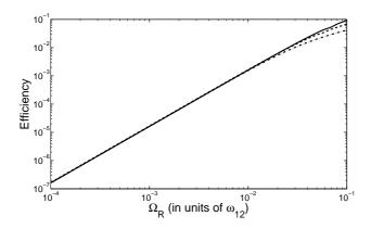
FIG. 10: Quantum efficiency versus the corresponding vacuum Rabi frequency at the voltage  $eV=E_{12}$ . The three lines are obtained with different values of the coherence damping coefficients:  $\Gamma_X=\Gamma_Y=0.1\omega_{12}$  (solid line),  $0.05\omega_{12}$  (dashed line) and  $0.025\omega_{12}$  (dashed-dotted line).  $E_{12}=150 \mathrm{meV}$ .
