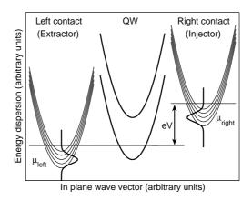
FIG. 2: Same as in Fig. 1, but with an applied voltage bias. Here, the left contact acts as an electronic extractor, while the right one is the injector. In the quantum well, non-equilibrium steady-state populations can be established in the two subbands.
