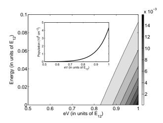
FIG. 6: Same as in Fig. 5, but for the second subband. Inset: the integrated density of electrons in the second subband versus voltage.
