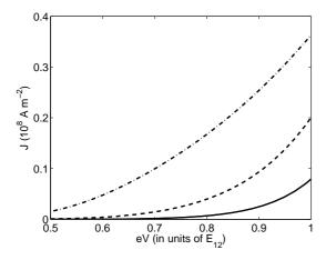
FIG. 3: Current density versus applied voltage for different values of the intersubband transition energy:  $E_{12} = 50 \text{meV}$ , (dashed-dotted line), 100 meV (dashed line) and 150meV (solid line). Other parameters can be found in the text.
