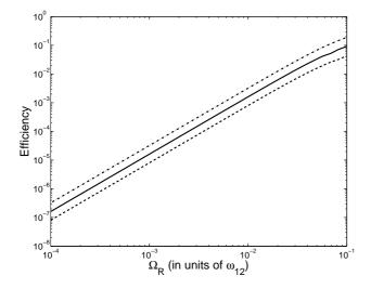
FIG. 11: Quantum efficiency versus the corresponding vacuum Rabi frequency at the voltage  $eV=E_{12}$ . The three lines are obtained with different values of the non-radiative relaxation rate:  $\frac{1}{\tau}=0.01\omega_{12}$  (dashed line),  $0.005\omega_{12}$  (solid line) and  $0.0025\omega_{12}$  (dashed-dotted line).  $E_{12}=150 \mathrm{meV}$ .
