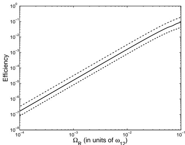
FIG. 11: Quantum efficiency versus the corresponding vacuum Rabi frequency at the voltage  $eV = E_{12}$ . The three lines are obtained with different values of the non-radiative relaxation rate:  $\frac{1}{\tau} = 0.01\omega_{12}$  (dashed line),  $0.005\omega_{12}$  (solid line) and  $0.0025\omega_{12}$  (dashed-dotted line).  $E_{12} = 150\text{meV}$ .
