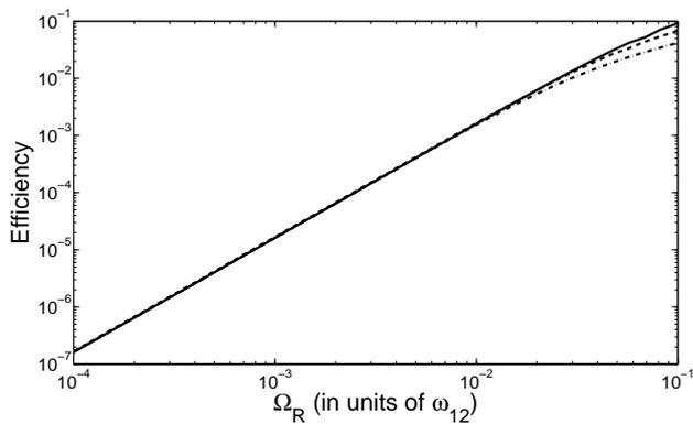
FIG. 10: Quantum efficiency versus the corresponding vacuum Rabi frequency at the voltage  $eV = E_{12}$ . The three lines are obtained with different values of the coherence damping coefficients:  $\Gamma_X = \Gamma_Y = 0.1\omega_{12}$  (solid line),  $0.05\omega_{12}$  (dashed line) and  $0.025\omega_{12}$  (dashed-dotted line).  $E_{12} = 150\text{meV}$ .
