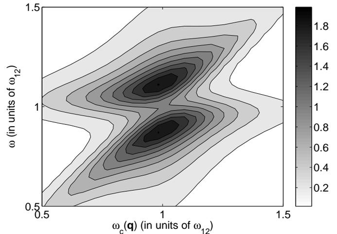
FIG. 8: Contour plot of the electroluminescence (arb. units) as a function of the bare cavity photon energy  $\omega_c(q)$  and of the emission frequency  $\omega$  for an applied voltage  $eV = 0.5E_{12}$ . The anticrossing of the two intersubband polariton branches is apparent in electroluminescence spectra.
