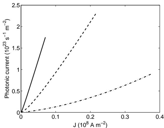
FIG. 4: Photonic current density versus electronic current for different values of the intersubband transition energy:  $E_{12} = 50\text{meV}$ , (dashed-dotted line),  $100\text{meV}$  (dashed line) and  $150\text{meV}$  (solid line). Same parameters and range of applied voltages as in Fig. 3.
