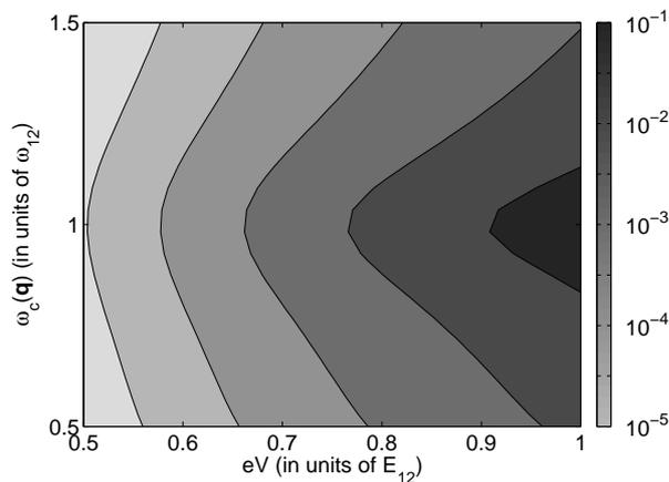
FIG. 7: Contour plot of the photon occupation (log scale) versus the applied voltage and the energy of the bare cavity photon mode.
