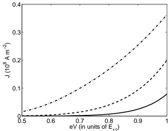
FIG. 3: Current density versus applied voltage for different values of the intersubband transition energy:  $E_{12} = 50\text{meV}$ , (dashed-dotted line),  $100\text{ meV}$  (dashed line) and  $150\text{meV}$  (solid line). Other parameters can be found in the text.
