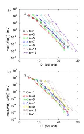
FIG. 3: (color online) a) Maximum of error made on the calculation of the potential at the position of the atoms of the central unit cell. D = n' + 2l - 2 is the width of the sets of charges in each crystallographic direction, where n' is the width of the central zone where the charges have their nominal values. l is the order of the first non zero momenta of the cell  $C_l$  used to construct the set of charges. b) Maximum of error made on the calculation of the difference of potential.
