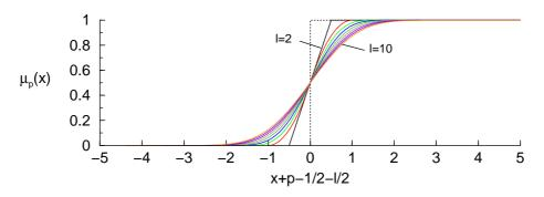
FIG. 2: (color online) Renormalization of the charges at the "left" edge of a crystal fragment, obtained for values of l ranging between 2 and 10. The origin of the abscises corresponds to the position of the edge obtained when using the original cell  $C_0$  (dotted line).
