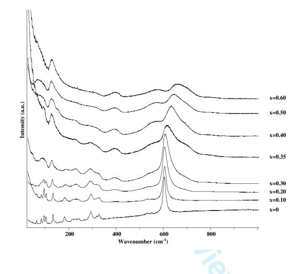
Fig. 2. Raman spectra of  $Ba_2In_{2-x}Sn_xO_{5+x/2}$  phases with x = 0, 0.1, 0.2, 0.3, 0.35, 0.4, 0.5, 0.6.
