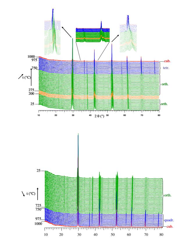
Fig. 4. High temperature X-ray diffraction data for  $Ba_2In_{1.9}Sn_{0.1}O_{5.05}$  upon a) heating and b) cooling.
