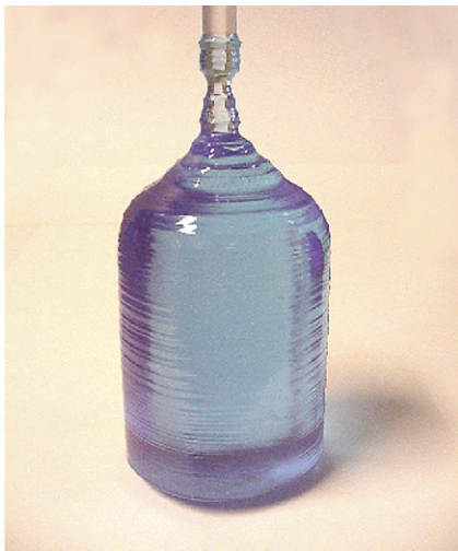
Fig. 1. A picture of a 5% Nd:YCOB crystal, grown by using Czochralski technique. Its dimensions reach 50 mm in diameter and 120 mm in length.
