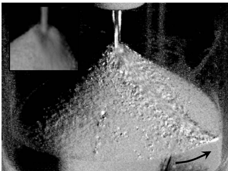
FIG. 4. Moving grains in the continuous river regime. The figure is the difference between two pictures of a continuous river separated by 0.15 s (the river was revolving around the pile at approximately 0.1 turns/s). This difference is superimposed with the first of these two pictures. The arrow indicates the direction of the revolution of the river around the pile. The inset shows a raw picture of the crater, at the upper end of the pile.
