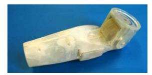
Fig. 8. Picture of the body part of the prosthesis with the elbow: use of Stereolythography process
