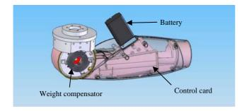
Fig. 7a. First view of the central structure of the prosthesis
