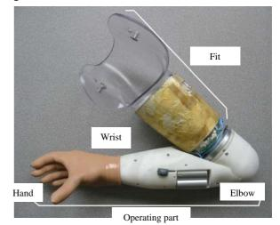
Fig. 10. The prosthesis of upper limbs developed
