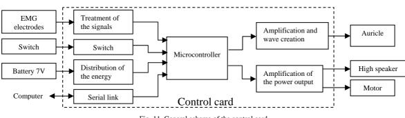
Fig. 11. General scheme of the control card
