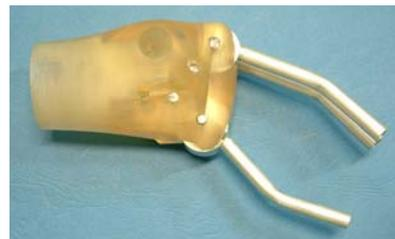
Fig. 9. The standard three legs grip hand used
