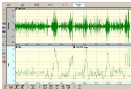
Fig. 12. EMG signal directly emitted by the patient's muscles and the treated signals
