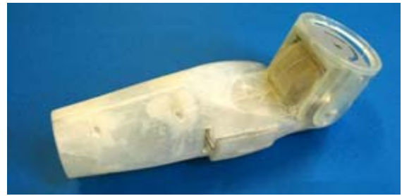
Fig. 8. Picture of the body part of the prosthesis with the elbow: use of Stereolithography process
