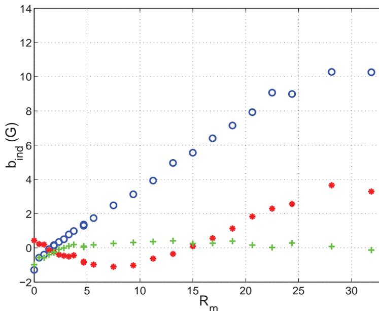
*Fig. 5.* Response to a transverse applied field in the case of two counter-rotating discs (the same configuration as in Fig. 3). The externally applied field  $B_0 = 9$  G is perpendicular to the rotation axis. The induced magnetic field  $\mathbf{b}_{ind}$  is measured in the mid plane, at a distance of 4 cm from the rotation axis. Its 3 components are plotted vs the magnetic Reynolds number  $Rm$ : (○) axial component  $b_x$ , (\*) transverse component  $b_y$ , (+) vertical component  $b_z$ .
