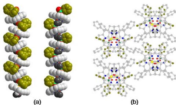
**Figure 3.** (a) Two different views in CPK of one  $[\mathbf{1}.\text{EtOH}]_\infty$  supramolecular chain. Light gray, C porphyrin; dark gray, C ethanol; dark green, C Ph on the phosphorus atom. (Ph *meso* and hydrogen atoms, except (O5)H, omitted for clarity). (b) View of the crystal packing along the  $c$  axis (hydrogen atoms, except (O5)H, are omitted for clarity).
