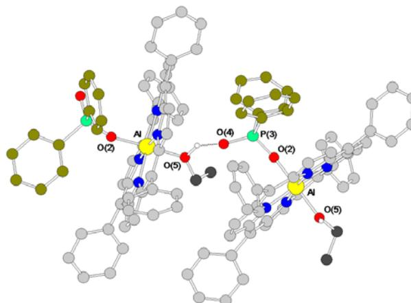
Figure 2. X-ray structure of [1.EtOH]<sub>n</sub> supramolecular chains. Light gray, C porphyrin; dark gray, C ethanol; dark green, C Ph on P(3). Hydrogen atoms, except (O5)H, are omitted for clarity.
