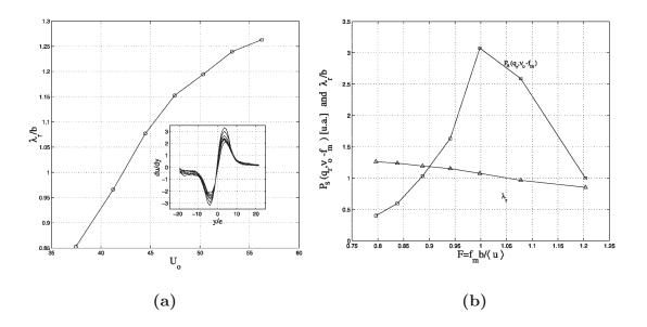
Fig. 10. (a) Evolution of the normalized resonant wavelength  $\lambda_r = 2\pi/q_r$  with the free stream velocity  $U_o$  for a forced wake ( $\zeta_m = 0.3 \text{ mm}, f_m = 10 \text{ Hz}$ ). (b) Evolution of the normalized resonant scattered pressure amplitudes ( $\sqcup$ ) and resonant wavelengths ( $\triangle$ ) with the dimensionless parameter  $F = f_m b/\langle u \rangle$ .
