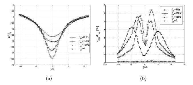
Fig. 6. Systematic effect of forcing frequency on the wake behavior (x/e = 79.4) at constant amplitude  $\zeta_m = 0.3$  mm and Reynolds number  $Re_b = 1185$ . (a) Mean velocity profiles  $\overline{u}/U_o$  and (b) velocity fluctuations  $u'/U_o$ . Note that the free wake behavior is indicated by a  $\sqcup$  ( $f_m = 0$  Hz).
