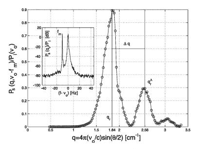
Fig. 8. Ultrasound scattering by the forced wake (forcing amplitude, frequency and Reynolds number are:  $\zeta_m = 0.3$ , mm,  $f_m = 10$  Hz,  $Re_b = 10^3$  respectively). We display the normalized amplitude of the scattered pressure as a function of the scattering wave vector q. The spatial resonance is obtained at  $q = q_r$  ( $\nu_o = 19.25$  kHz). The subplot shows the corresponding power spectrum of scattered pressure, where a Doppler peak is found at  $f - \nu_o = f_m$ .
