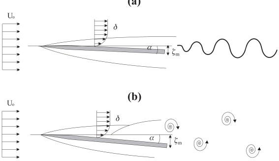
Fig. 1. Expected periodic patterns on a modulated wake through a periodic forced oscillation of the trailing edge of a thin flat plate. (a) Wavy wake for small forcing amplitude  $\zeta_m$ , (b) Large scale vortex shedding for higher forcing amplitude  $\zeta_m$ .
