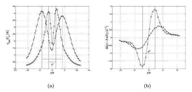
Fig. 5. Wake forcing at two different frequencies  $f_m = 5$  ( $\circ$ ) and  $f_m = 14$  ( $\sqcup$ ) Hz with same amplitude  $\zeta_m = 0.3$  mm and Reynolds number  $Re_b = 1185$ . (a) The velocity fluctuations  $u'(y)/U_o$  (x/e = 79.4) and (b) An estimation of the wake vorticity  $\Omega(y)$ . We indicate the increased cross stream scale of wake velocity fluctuations ( $\Delta^u$ ) and vorticity ( $\Delta^\Omega$ ) with the forcing frequency.
