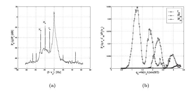
Fig. 12. Another example of higher harmonics production by a non linear wake. Forcing amplitude, frequency and Reynolds number are:  $\zeta_m = 0.3$ , mm,  $f_m = 10$  Hz,  $Re_b = 1.5 \times 10^3$  respectively. (a) Power spectrum of scattered pressure showing three Doppler peaks associated to the fundamental, first and second harmonics. (b) Spatial scales associated to the fundamental ( $\circ$ ), first ( $\sqcup$ ) and second harmonics ( $\triangle$ ).
