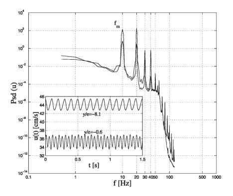
**Fig. 4.** Forced wake behavior from hot wire measurements. Forcing with amplitude  $\zeta_m = 0.3 \text{ mm}$  at  $f_m = 10 \text{ Hz}$  and Reynolds number  $Re_b = 1185$ . Power spectral density computed at two cross stream sites, y/e = -0.6, -8.1. The subplot shows typical velocity recordings at those positions.
