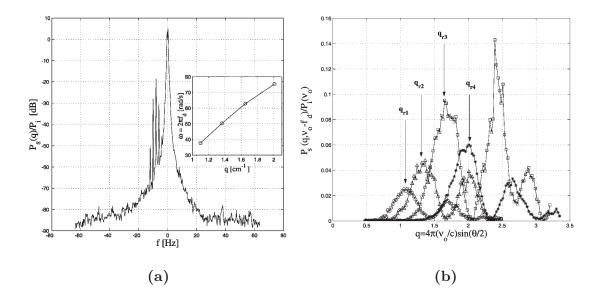
**Fig. 13.** Wake modulation at two forcing frequencies  $f_m^1 = 8, f_m^2 = 10$  Hz. ( $\zeta_m = 0.3$ mm,  $Re_b = 10^3$ ). (a) Power spectrum of scattered pressure showing four Doppler peaks (modes). The subplot showing their dispersion relation  $\omega(q)$ . (b) Spatial resonances at each Doppler peak, showing the presence of very different spatial modes in the wake. Doppler shifts are -6 Hz ( $\circ$ ), -8 Hz ( $\Delta$ ), -10 Hz ( $\sqcup$ ) et -12 Hz (\*).
