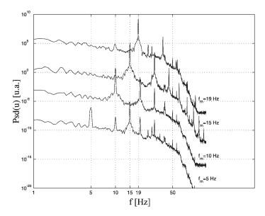
Fig. 7. Power spectra of wake velocity fluctuations at different forcing frequencies. Hot wire measurements performed at y/e = -8.1, x/e = 59.4 for a constant forcing amplitude  $\zeta_m = 0.3$  mm and Reynolds number of  $Re_b = 10^3$ .
