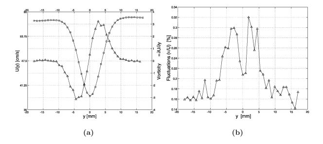
Fig. 3. Free wake behavior from hot wire measurements at x/e = 79.4 with  $\alpha = 0^{\circ}$  and  $U_o = 57$  cm/s. (a) Mean velocity profile ( $\sqcup$ ). We show also an estimation of the wake's vorticity ( $\triangle$ ) using first order numerical derivatives. (b) Wake velocity fluctuations.
