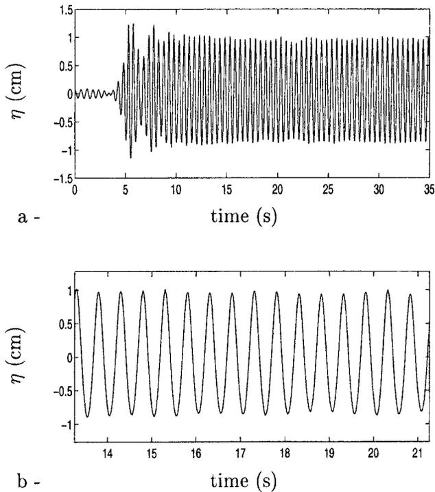
FIG. 9. Recording of a high-frequency wave group at 10 m from the wedge wave maker;  $f=2$  Hz,  $h_0=0.3$  m. (b) is a close-up of the recording plotted in (a) showing evidence of second-order contribution.
