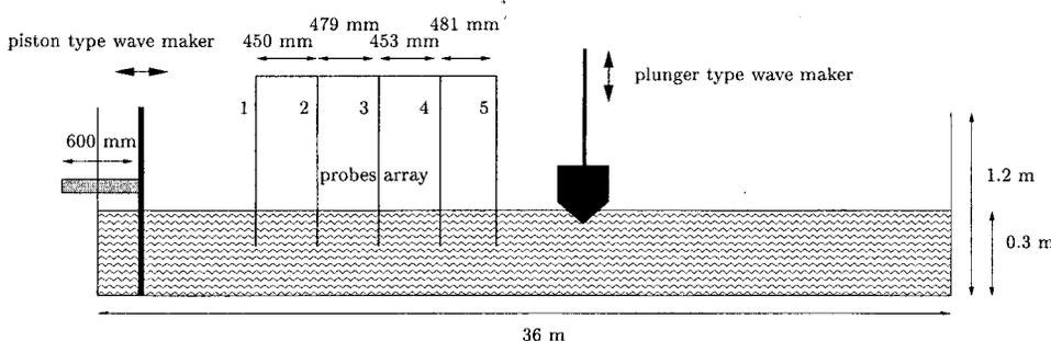
FIG. 8. Sketch and dimensions of the experimental equipment.
