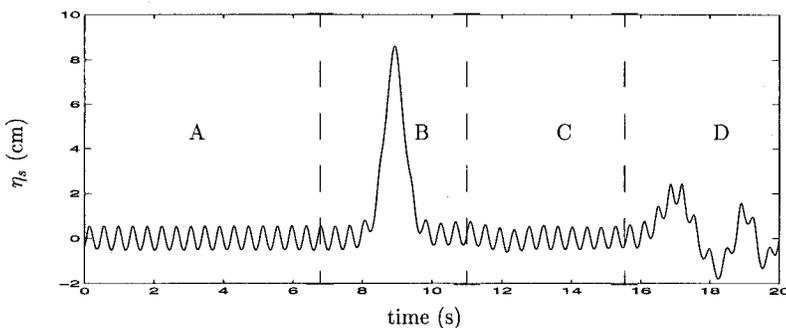
FIG. 10. Free surface elevation against time at 19.423 m from the piston wave maker; for the solitary wave  $A/h_0=0.3$  and the frequency of the short wave is  $f=2.5$  Hz ( $k_\infty=25.15$ ) for an amplitude of  $a_\infty=5.7$  mm ( $h_0=0.3$  m).
