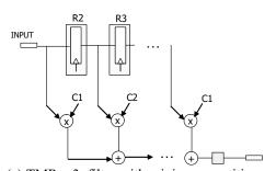
(c) TMR\_p3: filter with minimum partition Figure 4. TMR digital filter schemes used to evaluate the optimal logic partition of TMR
