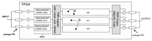
Figure 1. Triple Modular Redundancy (TMR) Scheme in the FPGA
