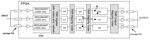
Figure 3. Triple Modular Redundancy (TMR) scheme with logic partition in the FPGA
