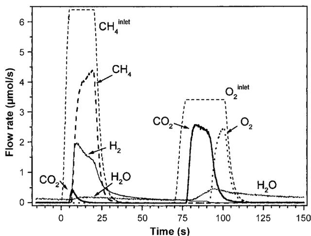
Fig. 1. Inlet and outlet gas concentrations obtained over 0.5 wt.% Pt/ $\text{CeO}_2$  tested at  $400\text{ }^\circ\text{C}$  by sequentially feeding a fixed bed reactor (4 mm i.d.) with methane, then helium and then oxygen.
