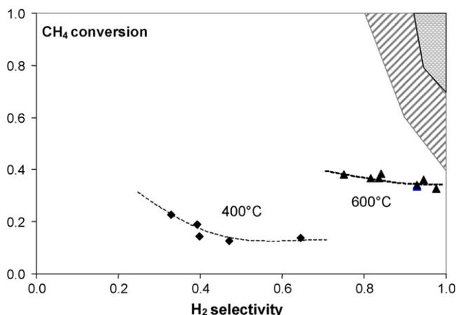
Fig. 5. Methane conversion vs. hydrogen selectivity data obtained with the sequential process at 400 and 600 °C and domains of performances for a conventional commercial POM process (dashed grey) and targeted for new process development (full grey) (unpublished data).
