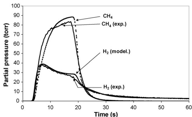
Fig. 3. Outlet gas concentrations obtained during step I over 5 wt.% Pt/CeO<sub>2</sub> catalyst at 400 °C compared with curves calculated according to the model [10].
