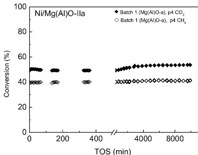
Fig. 3. Dry reforming of methane over Ni/Mg(Al)O II-a at 600 °C. Feed composition: CH<sub>4</sub>:CO<sub>2</sub>:H<sub>2</sub>:N<sub>2</sub> (%) = 10:30:10:50.
