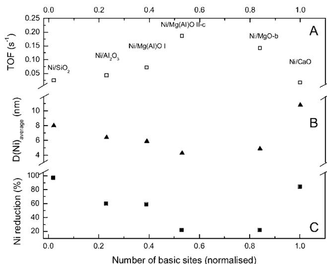
Fig. 6. (A) TOF after 1 h on-stream for all tested catalysts, (B) average Ni diameter and (C) degree of Ni reduction; all versus normalized concentration of basic sites from CO<sub>2</sub> TPD measurements. The values of Ni particle size and Ni reduction are those reported for reduced catalysts, see Table 2 (except for Ni/Mg(Al)O II, where Ni diameter after 2 min TOS is reported).
