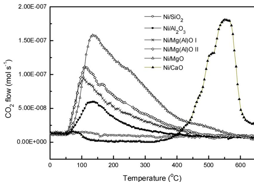
Fig. 4. CO<sub>2</sub> temperature-programmed desorption curves for the catalysts used in this study.
