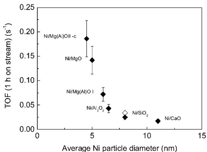
Fig. 5. TOF versus *D* after 1 h on-stream for all tested catalysts. The black markers were calculated using particle diameters from magnetic measurements (cf. Tables 1 and 2). The white marker was calculated by using the particle diameter estimated from TEM analysis for Ni/SiO<sub>2</sub>.
