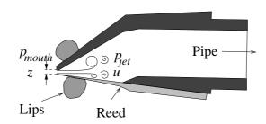
Fig. 1. Scheme of the embouchure of a clarinet.
