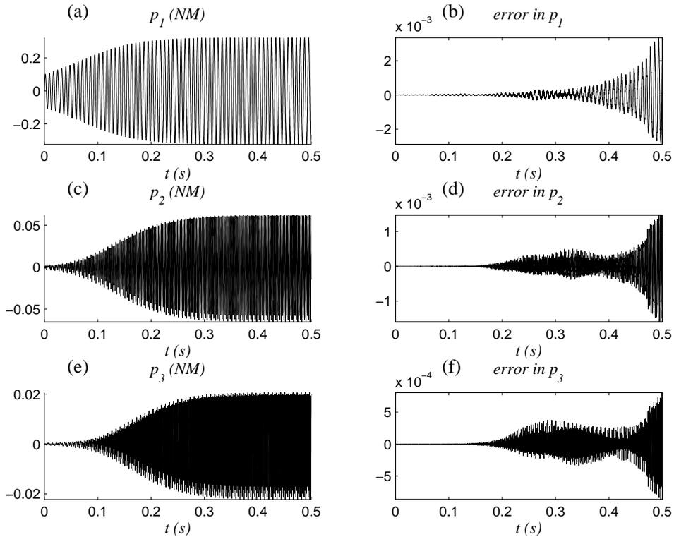
Fig. 5. First nonlinear mode: (a), (c) and (e) Time evolution of  $p_1$ ,  $p_2$  and  $p_3$  characterizing a modal motion according to the NM approach. (b), (d) and (f) Errors computed with a direct simulation of Eq. (11) and the same initial conditions as reference.
