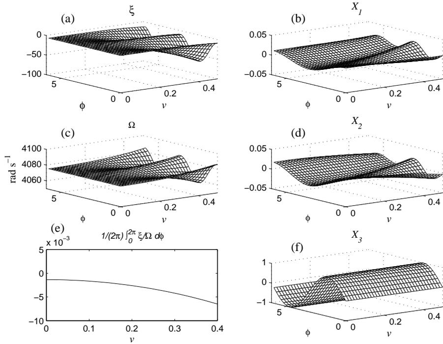
Fig. 11. Third nonlinear mode of the clarinet: (a) Damping function  $\xi$ , (b), (d) and (f) Surfaces for the three components of  $\mathbf{X}$ , (c) Instantaneous frequency  $\Omega$ , (e) The scalar function  $\langle \tau \rangle$ .
