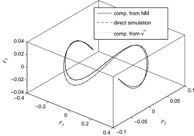
Fig. 6. First nonlinear mode: The limit cycle in the configuration space  $(p_1, p_2, p_3)$ . — Limit cycle computed from the nonlinear mode, - - - limit cycle according to direct simulation, ..... limit cycle computed from  $v^{**}$ .
