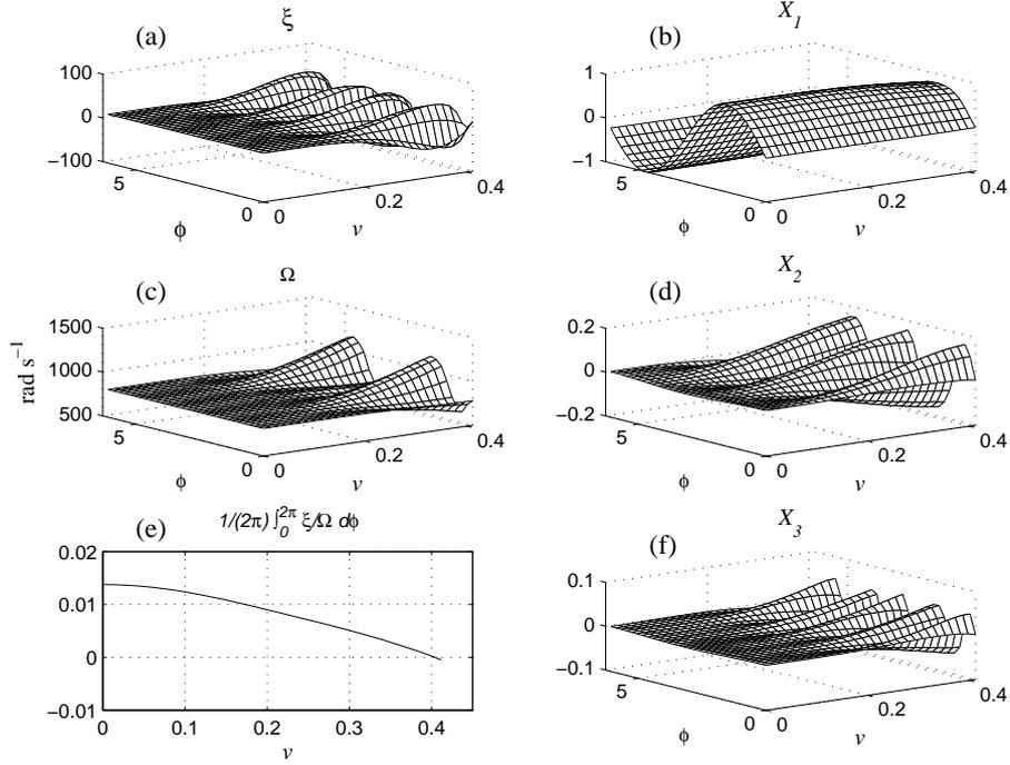
Fig. 3. First nonlinear mode of the clarinet: (a) Damping function  $\xi$ , (b), (d) and (f) Surfaces for the three components of  $\mathbf{X}$ , (c) Instantaneous frequency  $\Omega$ , (e) The scalar function  $\langle \tau \rangle$ , the zero of which indicates an estimate of the amplitude of the limit cycle.
