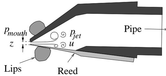
Fig. 1. Scheme of the embouchure of a clarinet.
