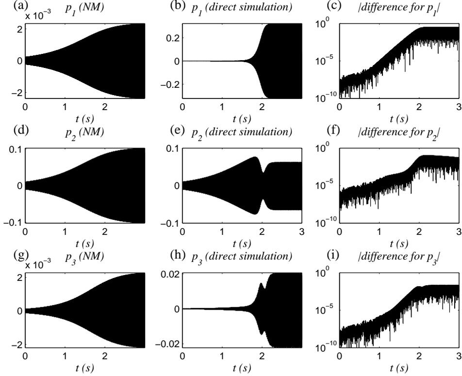
Fig. 10. Second nonlinear mode: (a), (d) and (g): Time evolution of  $p_1$ ,  $p_2$  and  $p_3$  characterizing a modal motion computed from the NM approach. (b), (e) and (h) Time evolution computed by direct simulation of Eq. (11) using the same initial conditions. (c), (f) and (i) Differences between solutions computed in the two different ways.
