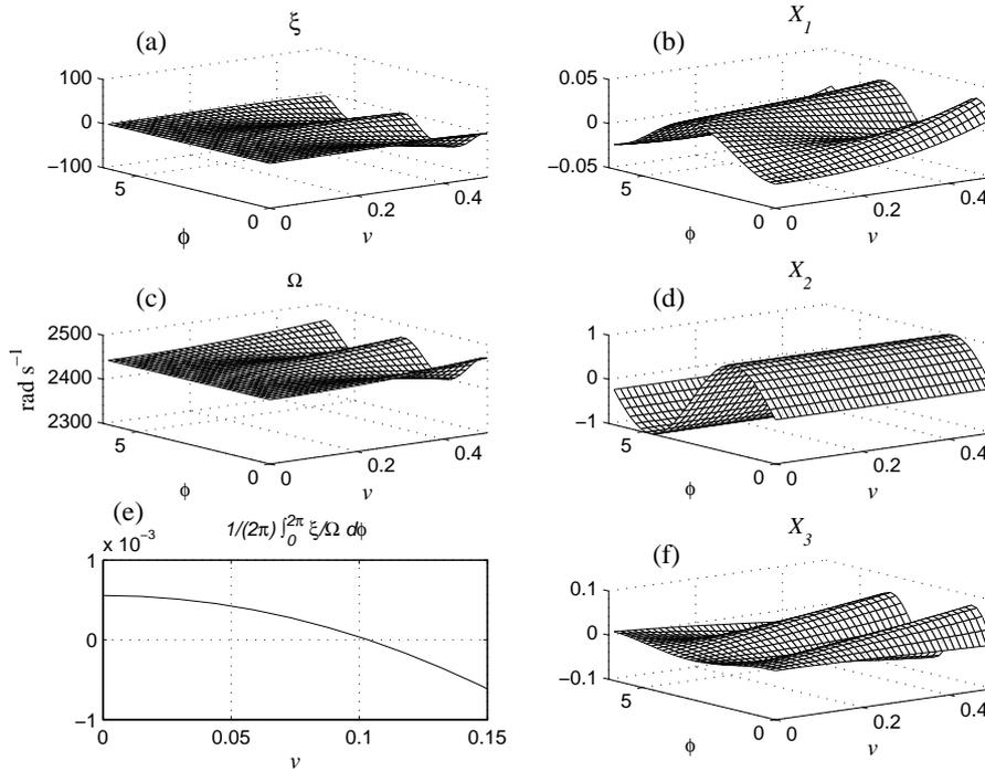
Fig. 7. Second nonlinear mode of the clarinet: (a) Damping function  $\xi$ , (b), (d) and (f) Surfaces for the three components of  $\mathbf{X}$ , (c) Instantaneous frequency  $\Omega$ , (e) The scalar function  $\langle \tau \rangle$ .
