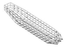
Figure 1: Example of a discrete distribution of tangential induced dipoles for a hull of a ship placed in a longitudinal inductor field.
