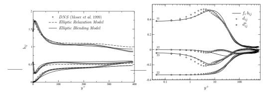
Figure 3. Comparison of Reynolds stress anisotropies predicted by the Elliptic Relaxation Model (13 equations) and the Elliptic Blending Model (8 equation)
