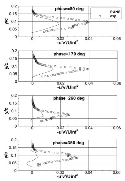
Figure 9. Turbulent shear stress profiles at x/c = 0.8 at four times during the oscillation cycle, for hump model with synthetic jet flow control.
