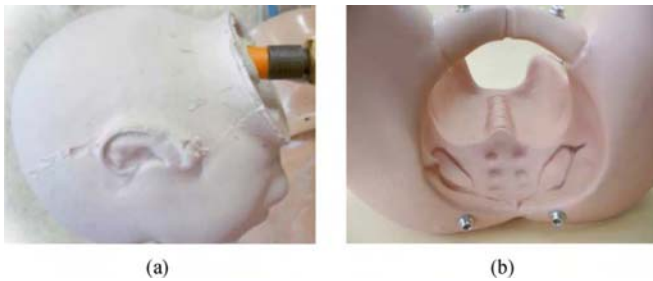
Fig. 2. The anthropomorphic models of the maternal pelvis and the fetal head. (a) The rebuilt silicone fetal head. (b) The pelvic model with its anatomical references: coccyx, sacrum, ischial spines, and pubis.
