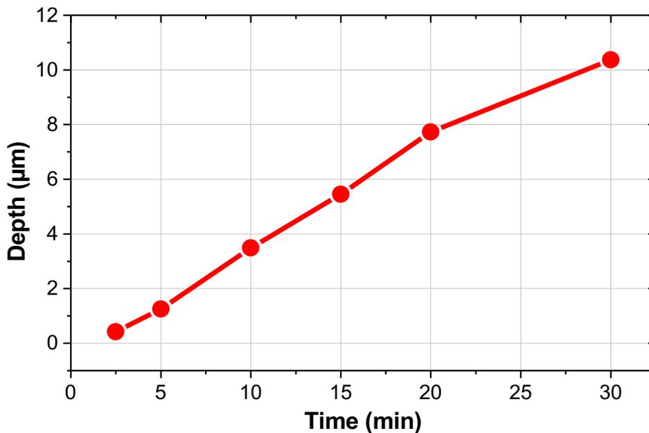
Fig. 1. Etching depth versus process duration
