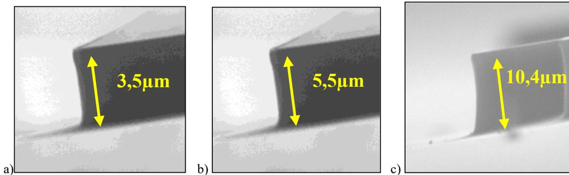
Fig. 2. SEM pictures of etching profile for a) 10, b) 15 and c) 30 minutes.
