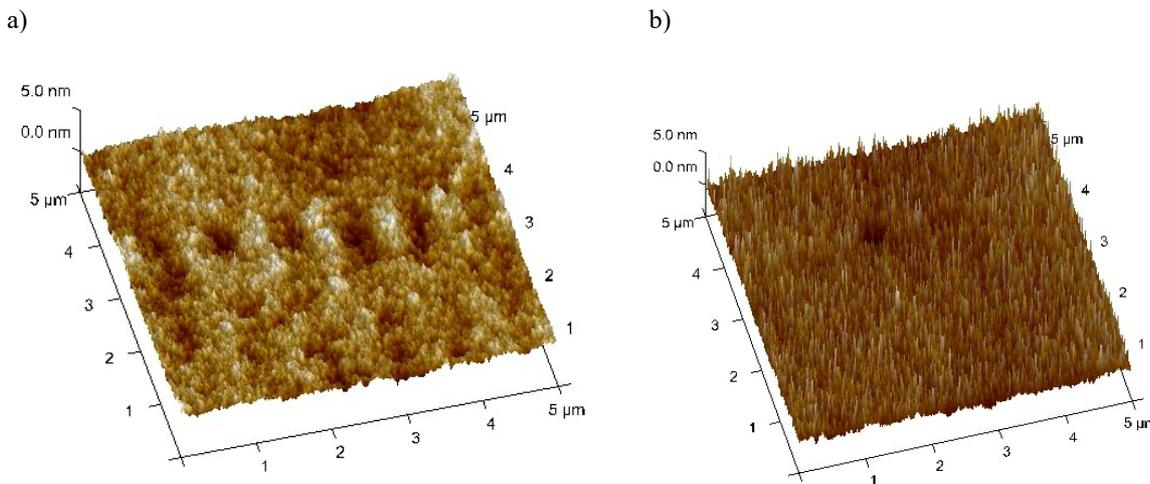
Fig. 3. AFM micrograph of etching process for a) 10 and b) 20 minutes
