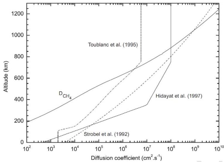
Figure 1: Eddy diffusion profiles - Hidayat et al. (1997) profile (solid line), Strobel et al. (1992) profile (dashed line) and Toublanc et al. (1995) profile (dot dashed line). The methane molecular diffusion coefficient profile is also included.
