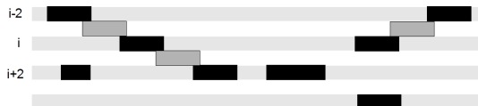
Fig. 8. The segments in dark gray represent the pixels interpolated thanks to the black neighboring segments
