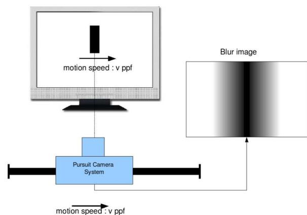
**Figure 1** MPRT-1000 Principle
