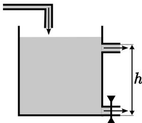
Fig. 1.1. One-tank system.
