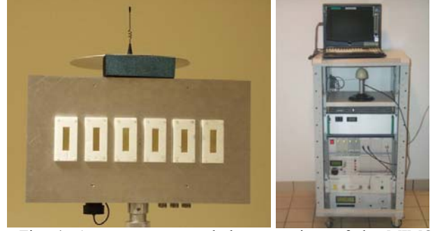
Fig. 4. Antennas array and the transmitter of the MIMO channel sounder.
