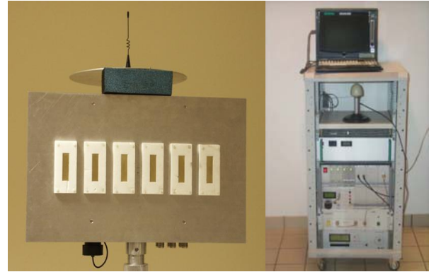
Fig. 7. Antennas array and the transmitter of the MIMO channel sounder.
