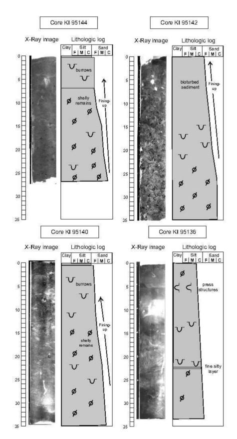
**Figure 4:** Radiographs (positives, mud in light grey and coarse sands in dark grey) and lithologic logs of four box cores sampled in June 1995 in the southern area of La Grande Vasière. Core KI\_95144 (latitude 46° 43′ 968, longitude 03° 08′ 178, water depth 100 m, station H); core KI\_95142 (latitude 46° 35′ 978, longitude 02° 58′ 567,
