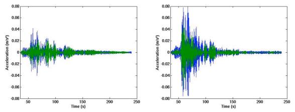
Figure 7: Comparison between recordings (blue) and modelling (green) of the Vallorcine earthquake at the top of the struture in the North (left) and East (right) directions
