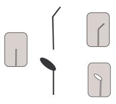
FIGURE 6. The magistral crack with a kink or cavity at the tip.
