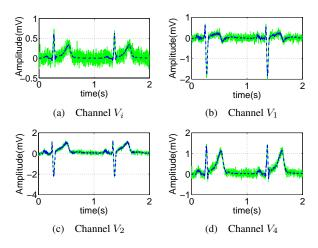
Figure 1. The noisy (solid line) and EKS denoised (dashed line) signals from some of the ECG channels.
