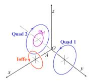
FIG. 2: Simplified scheme of the trap. After accomplishing evaporative cooling in the QUIC trap (Quad + Ioffe coils) centered at position A, the atoms are loaded into the dressed rf trap (Quad + Ioffe + rf coils). The current in the Ioffe coil is then slowly ramped down to zero for transferring the atoms into the dressed trap based on the quadrupole field of axis y (Quad + rf coils). The rf field polarization is aligned along the axis of the quadrupole.
