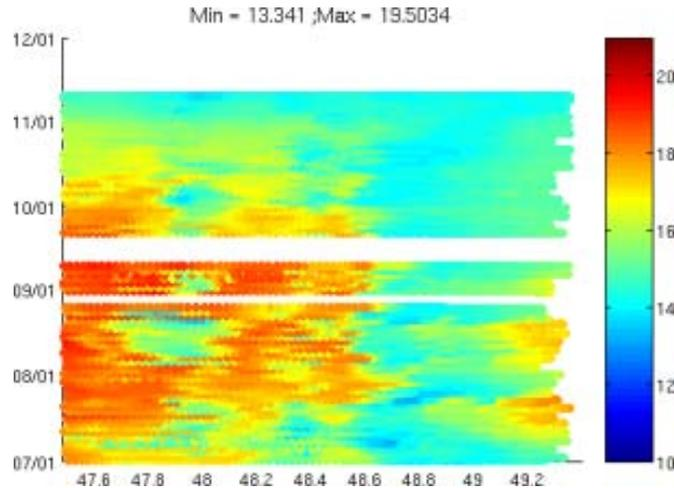
**Fig. 30. Sea surface temperatures (a) along the ferry trajectories (from [http://www.noc.soton.ac.uk/ops/ferrybox-2005/ferrybox\\_index\\_2005.php](http://www.noc.soton.ac.uk/ops/ferrybox-2005/ferrybox_index_2005.php)) (b) computed with MARS along the ferry trajectories**
