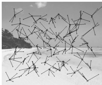
Fig 3 : A space-variant logarithmic ( R_0=2 ) retina for TheVibe. Note that the extent of the receptive fields increases with eccentricity. In particular, our mapping preserves overlap.
