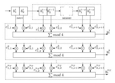
Fig. 1. ST trellis encoder with 4-PSK and  $n_T$  Tx antennas
