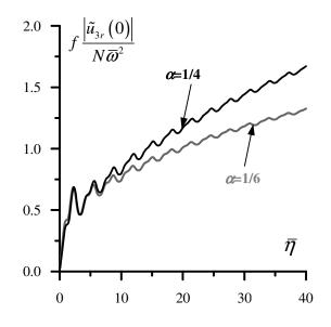
Dependence of the third harmonics amplitude  $|\tilde{u}_3(0)|$  of the shear wave at the surface on the normalized thickness  $\bar{\eta}$  of the granular layer for two different powers  $\alpha$  of the depth profile of sound velocity.
