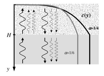
Reflection of plane acoustic waves from a layer of a granular material of thickness *H*. Axis *y* of the coordinate system is along the gravity direction  $\vec{g}$ . Assumed depth profiles of sound velocity *c* are presented for two power-law dependences on pressure  $p(c(p) \propto p^{\alpha}, \alpha = 1/6, 1/4)$ .
