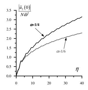
Dependence of the amplitude of the second harmonic  $|\tilde{u}_2(0)|$  of the longitudinal wave at the surface on the normalized thickness  $\overline{\eta}$  of the granular layer for two different powers  $\alpha$  of the depth profile of sound velocity.
