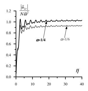
Dependence of the second harmonics amplitude  $|\tilde{u}_{2r}|$  of the longitudinal wave emitted into the substrate on the normalized thickness  $\overline{\eta}$  of the granular layer.
