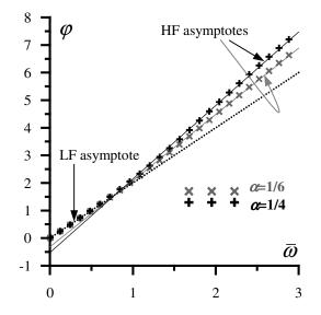
Dependence of the phase shift accumulated in reflection from a granular layer on dimensionless frequency  $\overline{\omega}$  of the acoustic wave. The curves corresponding to the general solution (26) are indicated by "×" and "+" symbols for  $\alpha = 1/6$  and  $\alpha = 1/4$ , respectively. The straight lines are low-frequency (see formula (27)) and high-frequency (see formula (28)) asymptotes.
