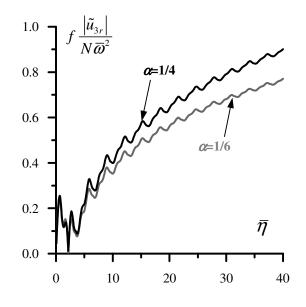
Dependence of the third harmonics amplitude  $|\tilde{u}_{3r}|$  of the shear wave emitted into the substrate on the normalized thickness  $\bar{\eta}$  of the granular layer.
