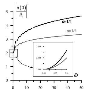
Dependence of the normalized surface displacement on the normalized frequency of the incident acoustic wave for two different profiles of in-depth velocity distribution  $(c(y) \propto y^{\alpha}, \alpha = 1/6, 1/4)$ .
