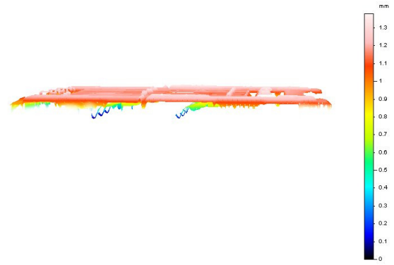
Fig. 10: 3D view of the SIM module, calculated from the image given in Fig. 9. Note that one single 2D bottom side measurement of the component is sufficient for generating this view.
