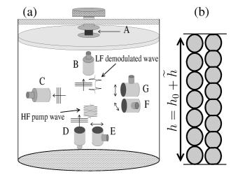
FIG. 1: (a) Diagram of the experiment. A is the force cell; B,C,D are longitudinal- and E,F,G are shear- transducers. Propagation lengths are 15-20 cm. (b) Two grain chains with essentially different static strains are sketched.
