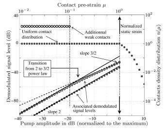
FIG. 3: Demodulated signal amplitude simulated for constant  $n(\mu)$  at  $0 \le \mu \le 1$  (squares) and in presence of localized weak fraction (circles) containing 60% of the total contact amount. The latter simulation provides clear transition  $2 \rightarrow 3/2$  in the slope at  $\varepsilon_p \ll \varepsilon_0$ .
