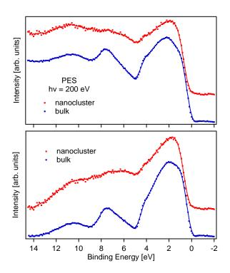
FIG. 1: PES valence band spectra (top) and secondary electron background corrected data (bottom) for a bulk crystal and 3.3 nm nanocluster sample. The spectra were acquired with a photon energy of  $h\nu = 200$  eV.
