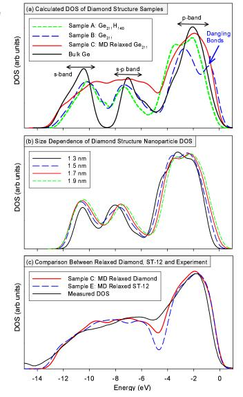
FIG. 3: (a) Predicted electronic DOS of the germanium nanoclusters listed in Table I, (b) calculated size dependence of the DOS for diamond structure nanoparticles, and (c) comparison of calculated diamond and ST-12 DOS with the measured DOS
