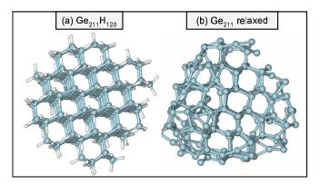
FIG. 2: Atomic structures of (a) Sample A,  $Ge_{211}H_{140}$  with a diamond structure core and (b) sample D,  $Ge_{211}$  with an MD relaxed structure.
