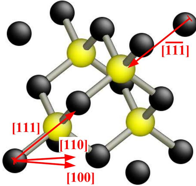
FIG. 1: Representation of the main crystallographic directions in  $\beta$ -SiC. Carbon atoms are drawn in black, and silicon atoms in light grey (yellow in the electronic version).
