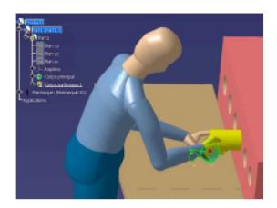
Manikin under Delmia<sup>™</sup> being controlled by IK.
