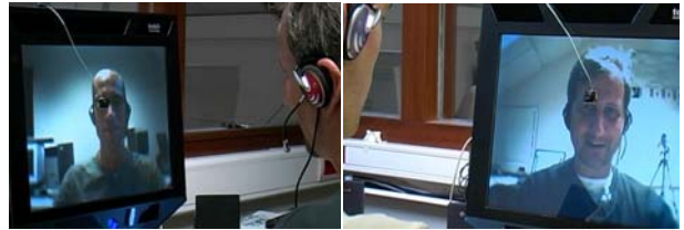
Figure 1: Experimental setup: In contrast to video phones this setup enables real size rendering of video image and eye contact, as the camera is placed on the screen. With additional audio transmission it is therefore very close to a scenario where interlocutors face each other across a table.
