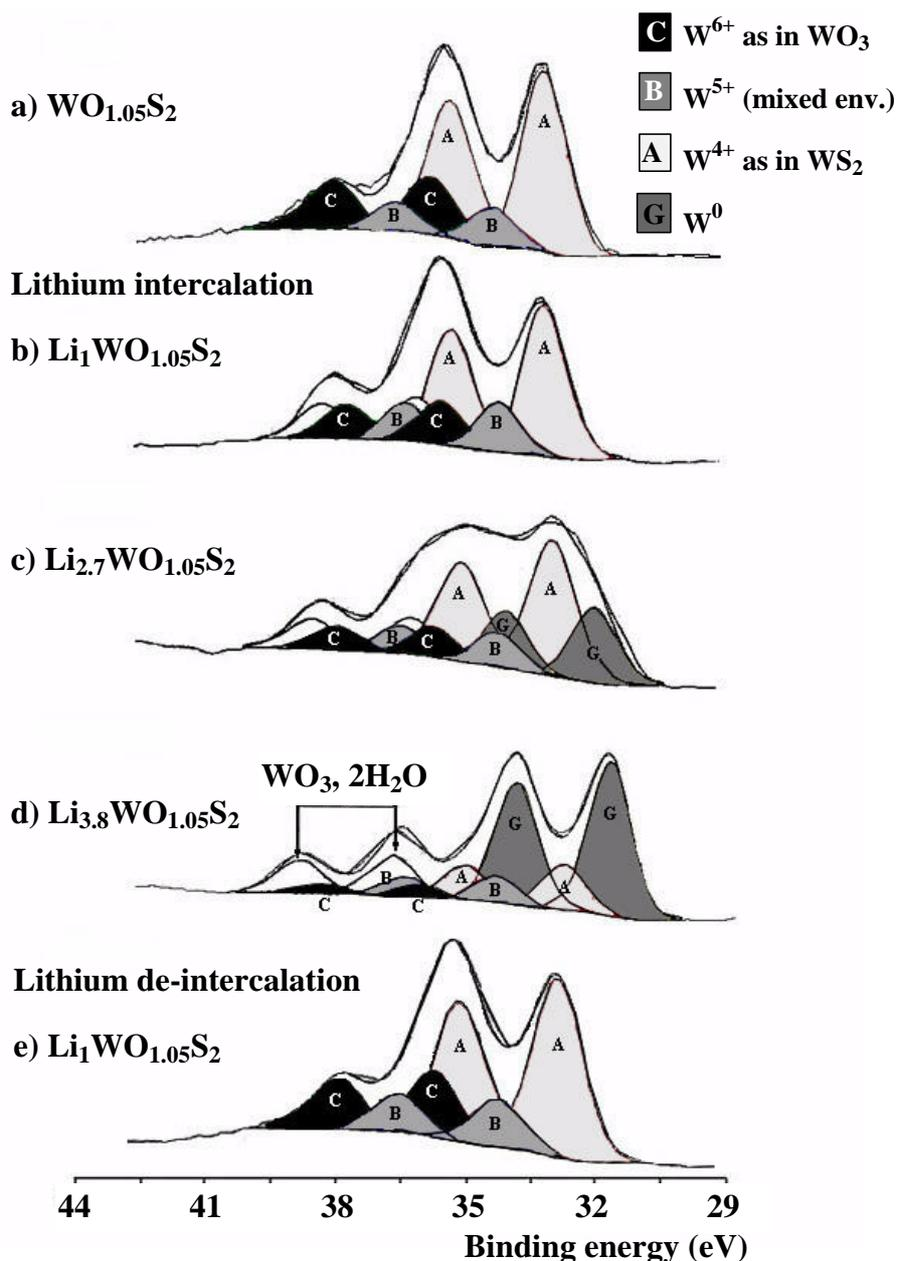
**Figure 5.** The XPS W4f peak of a  $\text{Li}_x\text{WO}_{1.05}\text{S}_2$  thin film at various stages of the first cycle. (a) starting material,  $x = 0$ , (b), (c) and (d) lithium intercalation, respectively at  $x = 1$ , 2.7 and 3.8, and (e) end of the charge,  $x = 1$ .
