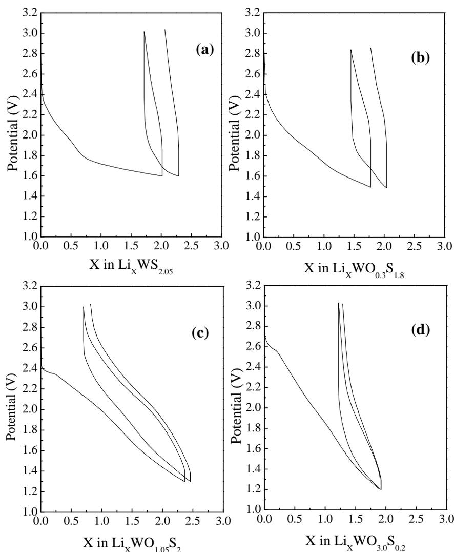
**Figure 1.** The 2 first cycles for different Li/LiAsF<sub>6</sub>, EMC 1M/WO<sub>y</sub>S<sub>z</sub> cells cycled at 3 μA/cm<sup>2</sup>. (a) WOS<sub>2.05</sub>, (b) WO<sub>0.3</sub>S<sub>1.8</sub>, (c) WO<sub>1.05</sub>S<sub>2</sub> and (d) WO<sub>3.0</sub>S<sub>0.2</sub>.
