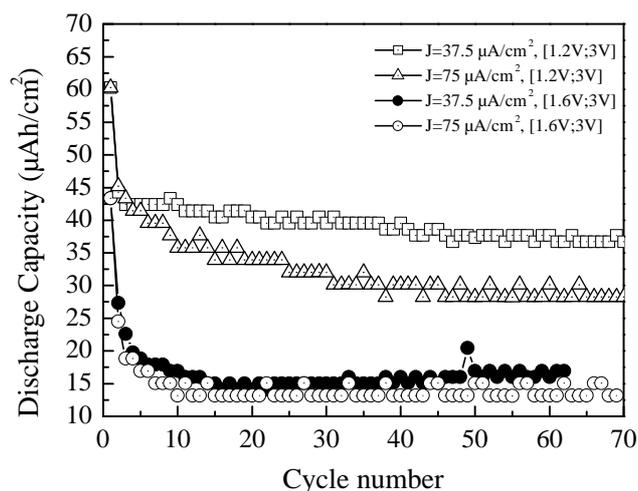
**Figure 3.** Discharge capacity vs cycle number for Li/LiAsF<sub>6</sub>, EMC 1M/WO<sub>1.05</sub>S<sub>2</sub> cells, at different potential windows and different current densities.
