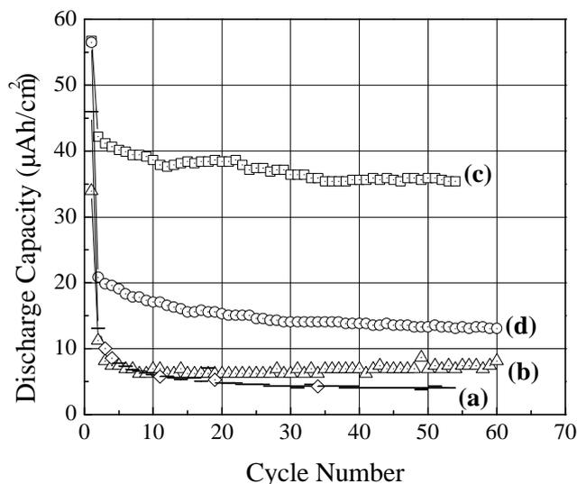
**Figure 2.** Discharge capacity vs cycle number for different Li/LiAsF<sub>6</sub>, EMC 1M/WO<sub>y</sub>S<sub>2</sub> cells cycled at 3 μA/cm<sup>2</sup>. (a) WOS<sub>2.05</sub>, (b) WO<sub>0.3</sub>S<sub>1.8</sub>, (c) WO<sub>1.05</sub>S<sub>2</sub> and (d) WO<sub>3.0</sub>S<sub>0.2</sub>.
