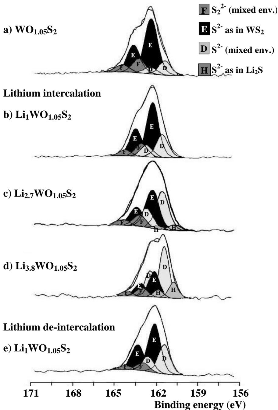
**Figure 6.** The XPS  $\text{S}2p$  peak of a  $\text{Li}_x\text{WO}_{1.05}\text{S}_2$  thin film at various stages of the first cycle. (a) Starting material,  $x = 0$ , (b), (c) and (d) lithium intercalation, respectively at  $x = 1$ , 2.7 and 3.8 and (e) end of the charge,  $x = 1$ .
