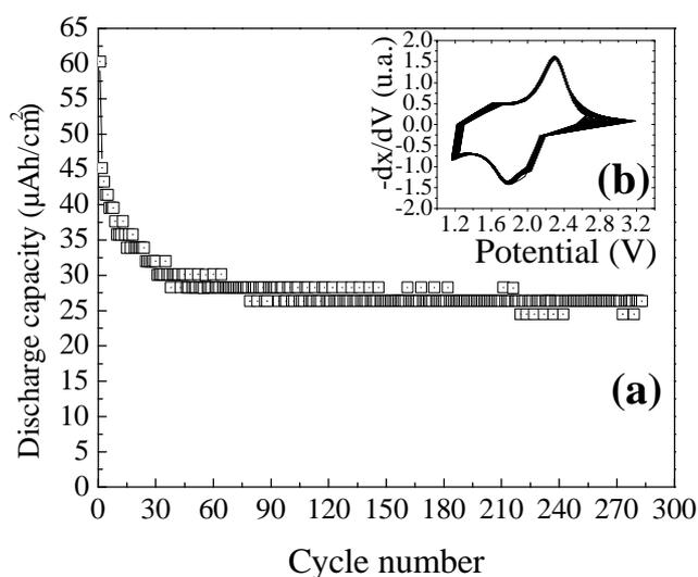
**Figure 4.** The behaviour of a Li/LiAsF<sub>6</sub>, EMC 1M/WO<sub>1.05</sub>S<sub>2</sub> cell cycled at 75 μA/cm<sup>2</sup> between 3.0 V and 1.2 V. (a) Discharge capacity vs cycle number and (b) incremental capacity derivative vs cell voltage between the 150th and 220th cycles.
