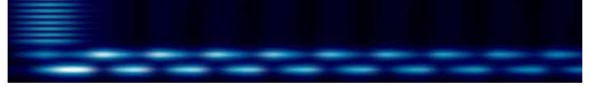
Figure 2: The two identical coupled waveguides of height 0.2 \lambda are excited using evanescent coupling : an incident beam with an incidence angle of 36,9 in a medium with \epsilon = 5 and \mu = 1 is used. The energy oscillates between the two guides and leaks out when it is in the upper guide, so that it decays exponentially.
