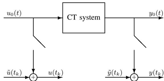
Fig. 1. CT system with noisy input/output data
