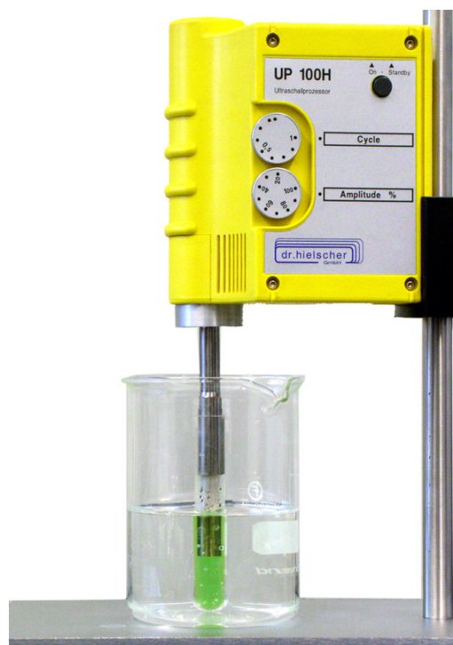
Picture 1 – 100W Setup for Feasibility Testing
