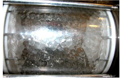
Fig. 2: Two-dimensional cylindrical subharmonic wave patterns (hexagons) under a sinusoidal forcing at frequency f_0 = 30 Hz, and amplitude d_0 = 0.29 mm leading to a 1.06g acceleration. Cylindrical container filled with 30 cl of ethanol.
