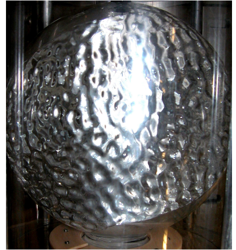
Fig. 3: Two-dimensional spherical subharmonic wave patterns under sinusoidal forcing at frequency f_0 = 30 Hz, and amplitude d_0 = 0.32 mm leading to a 1.16g acceleration. Spherical container filled with 20 cl of water.
